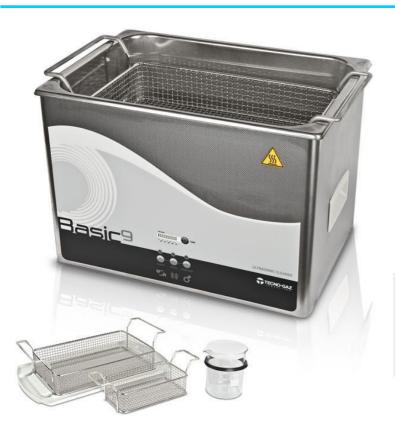
The ultrasonic tub is designed to wash instruments used in the medical, dental, cosmetic, veterinary fields of application and all those areas which require an ultrasonic washing. The cleaning device involving ultrasound (via cavitation) allows you to thoroughly clean places otherwise difficult to reach by manual cleaning, without any risk resulting from unsafe handling of contaminated instruments.
